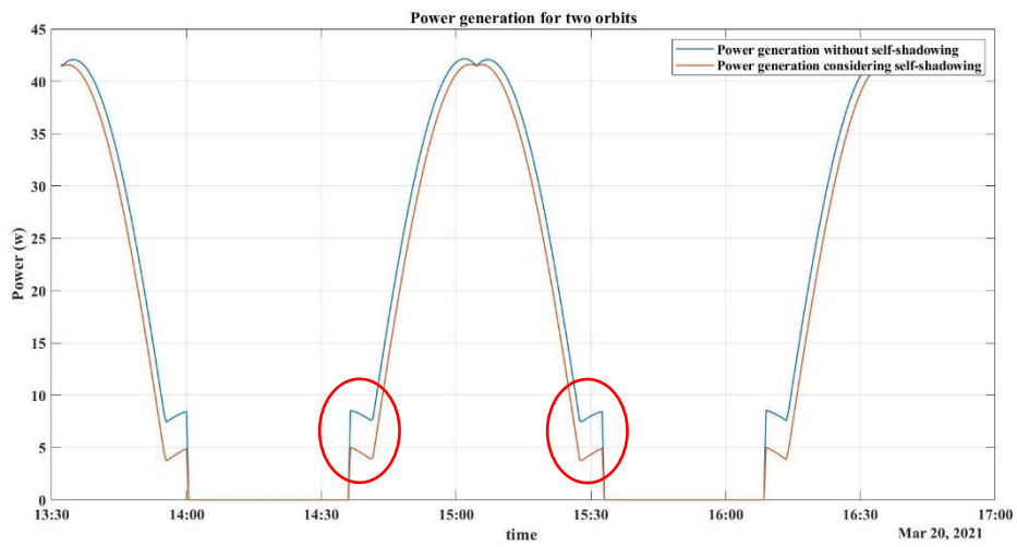
Figure 70: BM-DP-V-90 power generation in two orbits with considering the self-shadowing
