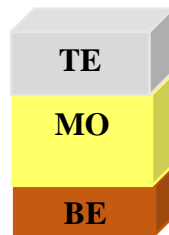
Figure 2.19: Memristor physical structure
