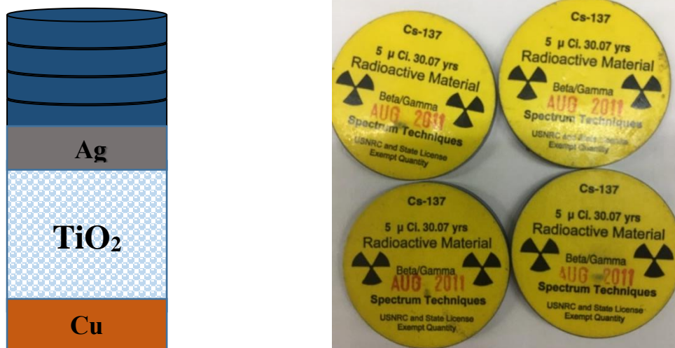
Figure 3.12: a) Experimental setup, b) Cesium-137 \gamma -ray with active diameter of 5mm, type-D, a radioactivity of 5\mu Ci and primary emitted photon energy of 662keV
