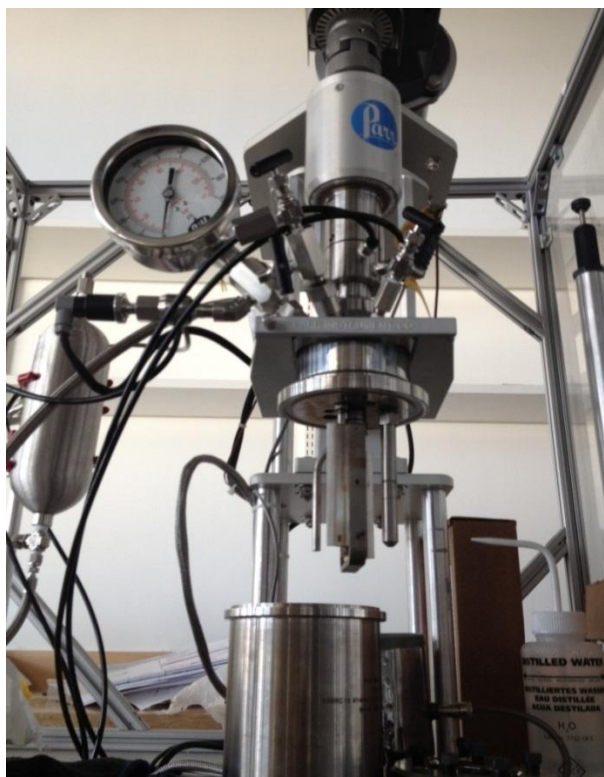
Figure 3-1. The reactor used for hydrothermal pre-treatment of salicornia biomass
